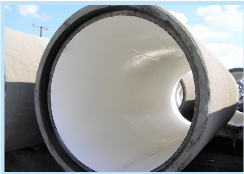
Plastic liner protects Concrete Pressure Pipe lining from acid generated from sewer gas.
