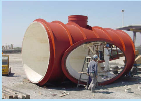
90° wye outlet fitting for 132" sewer pipe, with plastic liner.
