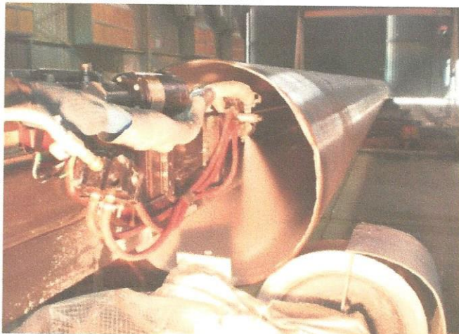
ABOVE ▲ This photo shows the application of liquid epoxy lining to the interior of a rotating steel water pipe. A similar process is used for polyurethane linings.
