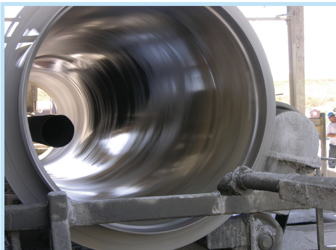
Centrifugal casting packs the aggregate into the lining, resulting in a smooth pipe interior.
