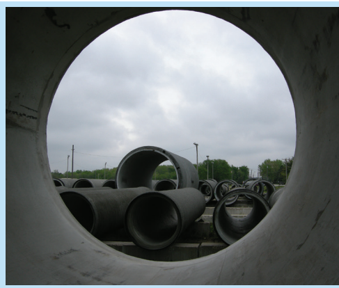
Concrete pressure pipe lining is produced either by centrifugal casting or, as for the lining in this picture, by vertical "wet-casting" against a smooth steel form.
