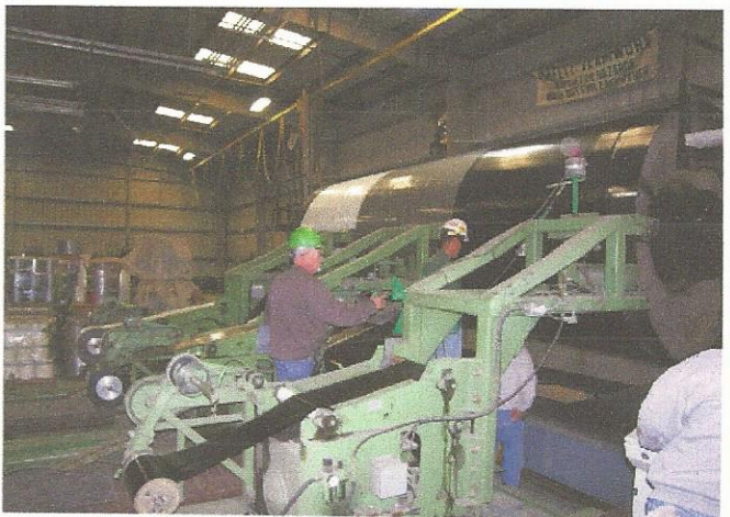
BELOW ▾ Application of a three-layer tape coating to steel water pipe.
