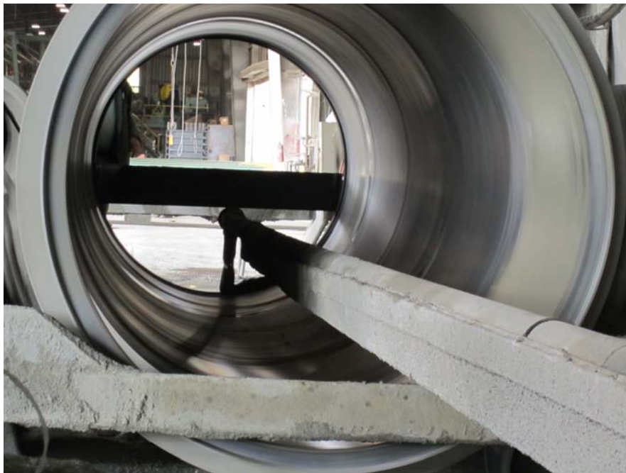
Photograph 1. Mortar lining manufacturing process.
