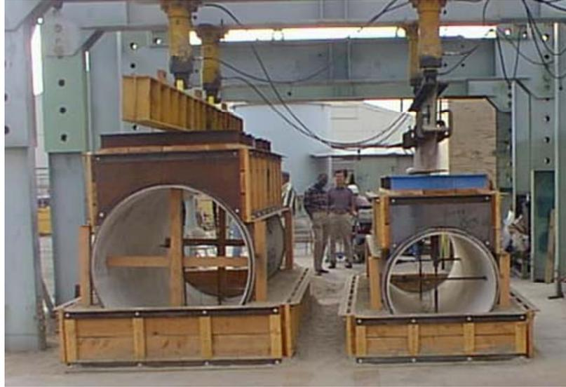
Figure 2. Set up for Sand-Bearing Load/ Deflection Tests
